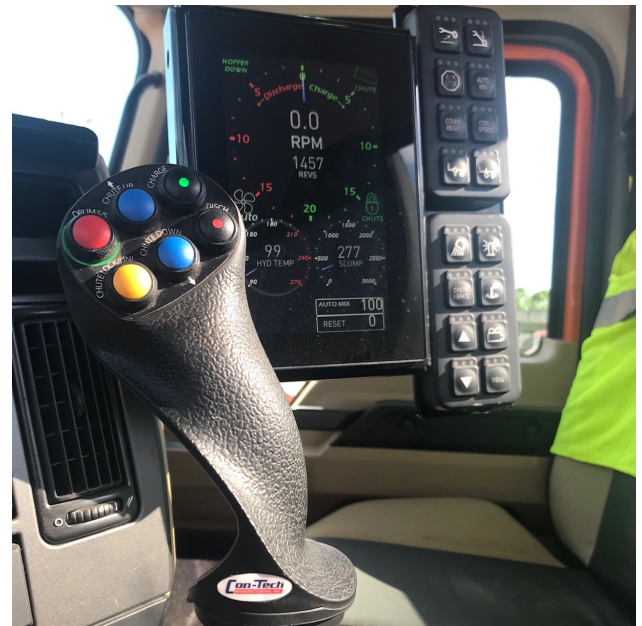
Joystick, LED screen and remote control in Con-Tech mixer.
