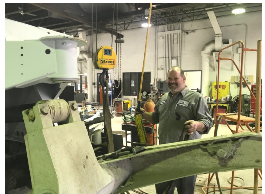
Senior Mechanic, Craig Ramey performing rear pedestal work and about to put a drum roller on truck #597.
